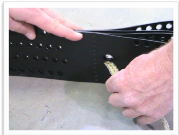
4. Pull the tendon through the tendon hole.
