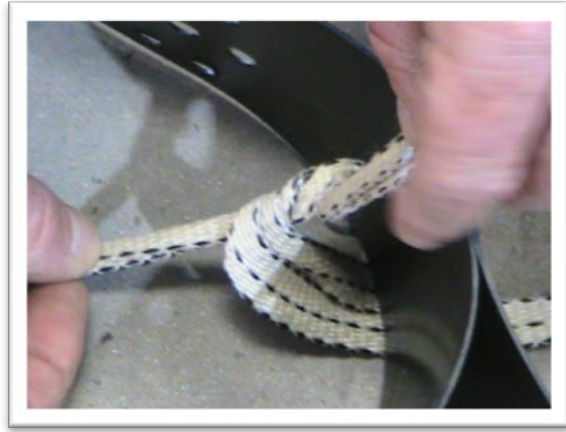
12. Pull on tendon loop until tight
