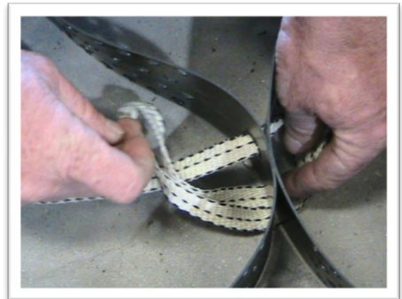
10. Feed loop over tendon.
